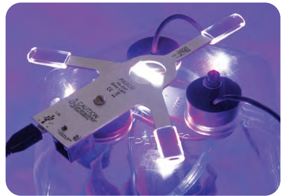
When connected to a //control.Node, the red and blue LEDs can be controlled using Blockly code, available in both SPARKvue and PASCO Capstone.
